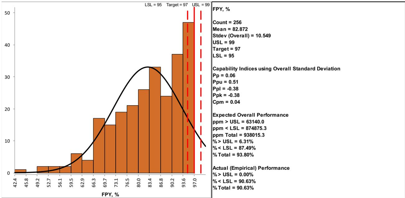
Figure 4. TC First Pass Yield manufacturing process capabilities
