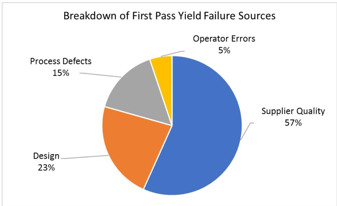
Figure 6. TC First Pass Yield failure sources
