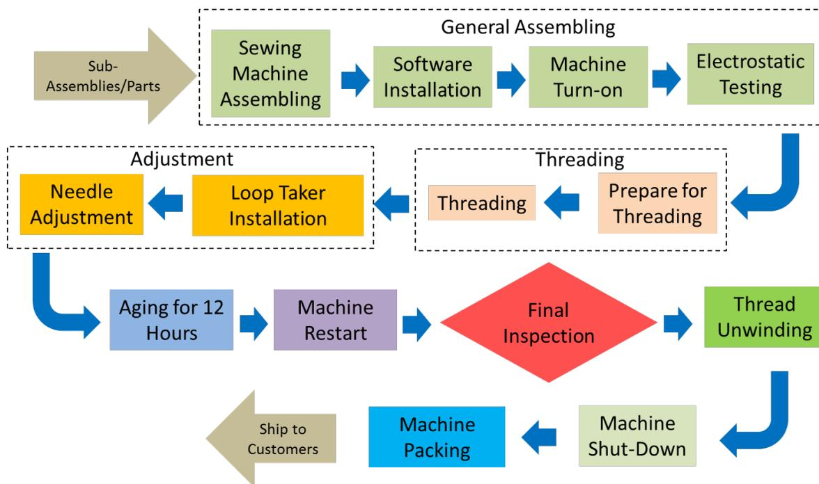
Figure 2. TC sewing machine manufacturing process flow
